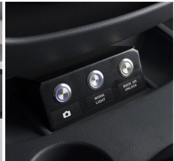
Control Panel For Locking & Lighting System
