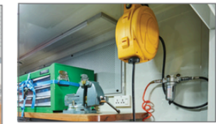
Air Hoses On Reel and Recoiled for Air-Operated Tools
